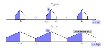
The resulting signal has sampling period MT/L = 3T/2. Note that aliasing was prevented by selecting the cutoff frequency  $min(\pi/2, \pi/3) = \pi/3$ .
