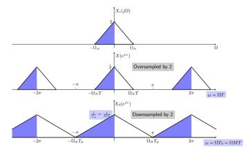
To obtain the spectrum we discrete time, we just need to use the change of variables  $\omega=\Omega T$  and  $\omega=\Omega T_d$
