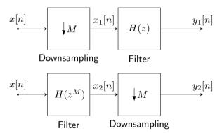
To move the filter before downsampling by M, we must stretch its frequency response by a factor of M:  $H(z^M) \xrightarrow{z=e^{j\omega}} H(e^{j\omega M})$ .
