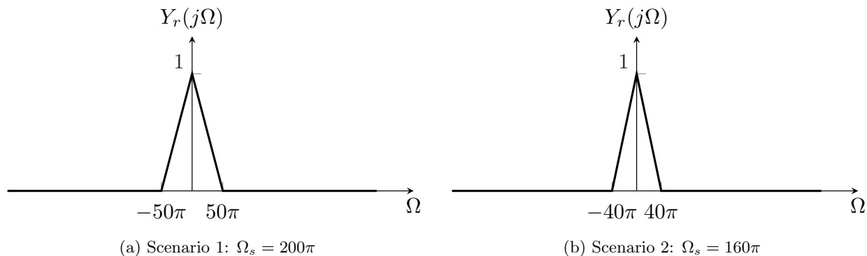
Figure 6: Output spectrum after reconstruction when (a) \Omega_s = 200\pi and (b) \Omega_s = 160\pi .
