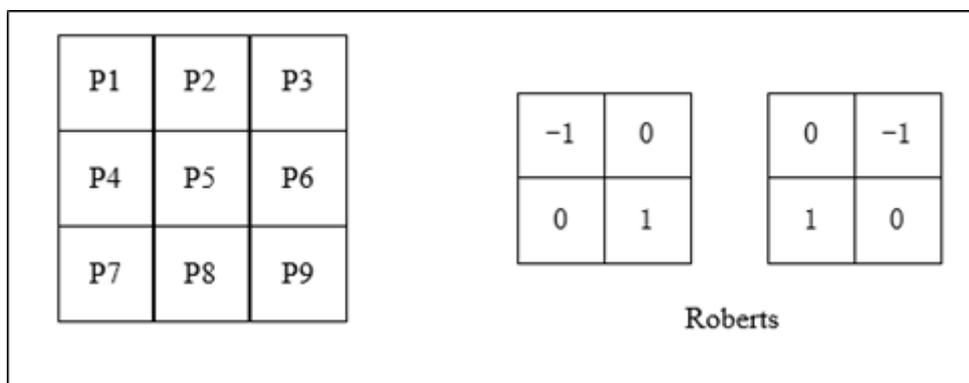
$$\begin{aligned} g_x &= \frac{\partial f}{\partial x} = P9 - P5 \\ g_y &= \frac{\partial f}{\partial y} = P8 - P6 \end{aligned} \quad (3)$$
